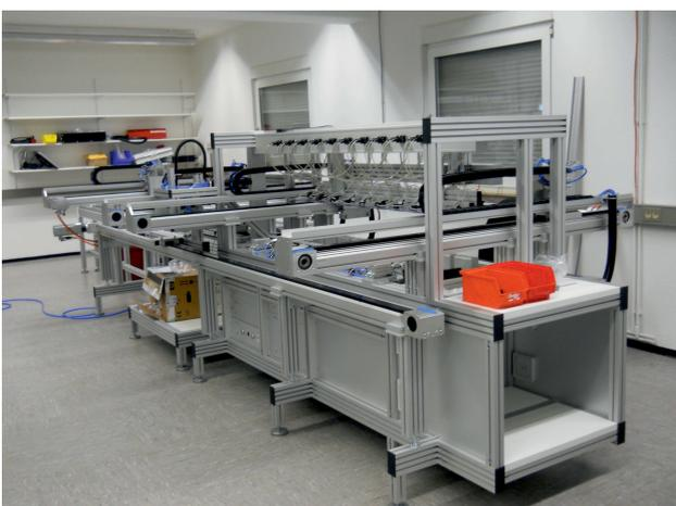
This highly customized project example shows a fully automatic test system for single-phase meters on 5 trays with 10 measuring positions each.
