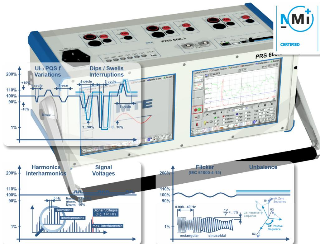
The PRS 600.3 is a combination of a three-phase Portable Reference Standard of class 0.02% and an IEC 61000-4-30 Class A compatible Power Quality Analyzer with 3 voltage and 3 current channels. The device is equipped with two 8.4" colors TFT displays based on touch screen operation. The Reference Standard is used to test single and three phase meters, instrument transformers and installations on site.
