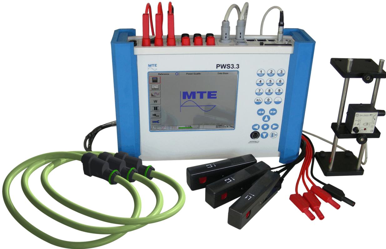
The PWS 3.3 is a combination of a three-phase Portable Working Standard of class 0.05% or 0.1% and an IEC 61000-4-30 Class A compatible Power Quality Analyzer with 3 voltage and 4 current channels.
