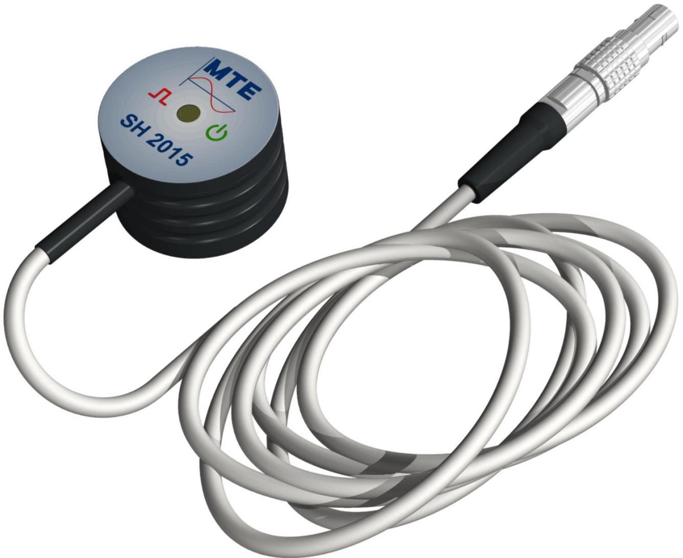
The photoelectric scanning head Type SH 2015 is especially designed to detect pulses from electronic meters. A permanent ring-magnet is built into the scanning head, thus enabling the SH 2015 scanning head to be magnetically attached to meters with built-in metal ring or magnet around the light emitting diode.
