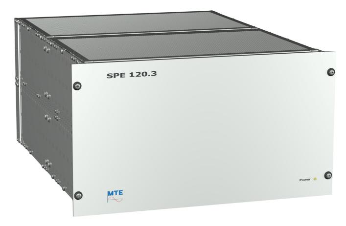
The SPE 120.3 is a three-phase computer controlled voltage and current source, designed for used in meter test systems and in the laboratory. It is in two performance steps with 300 VA and 600 VA output power available. The models are housed within a 19"-plug-in unit, 6 or 9 height modules, depending on output power.
