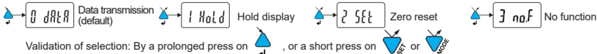
**Note:** a function can also be assigned via RS232 using the command <FCT + Function No.> (FCT 0...3)
