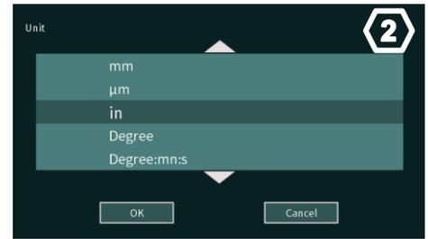
The choice of unit allows the definition of length, angle and customised units.
