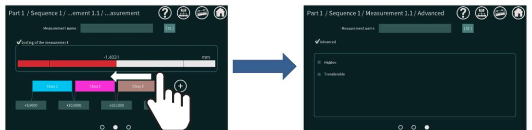
**Hidden option:** Allows the measurement on the measurement screen to be hidden
